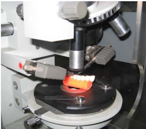
Fig.3. The method of laser micro spectral analysis is a method of punctual method of analysis, which allows to investigate small quantity of material, around 0.1 \mu\text{g} .
