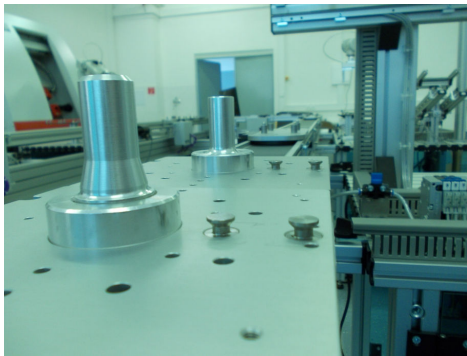
Fig. 11 Final product of Penholder in system iCIM 3000
