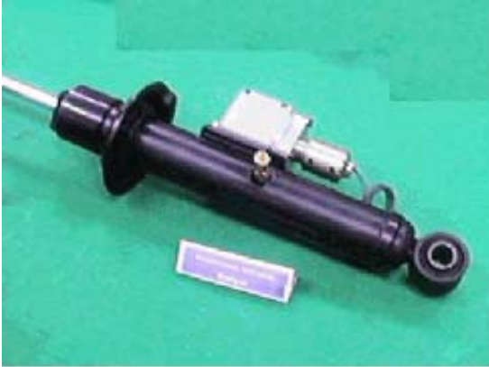
Fig. 10 Photograph of reverse continuous variable damper
