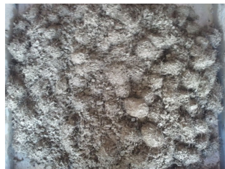
Fig. 4 Fiber ball Phenomenon (S44F1.25, S44V1.5, S51V1.5)
