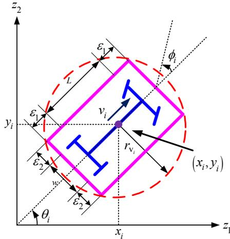
Fig. 1 Kinematic model of the car-like mobile robot
