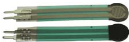
Fig. 20 0.2 Inch Interlink Force Sensing Resistor 400 Source: [25]
