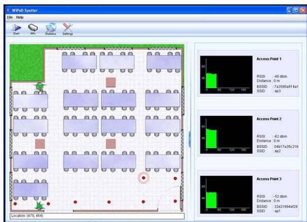
Fig. 1 WiPoD Spotter, wireless data collection and utility program
