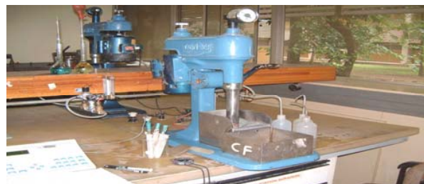
Fig. 4 Laboratory flotation machine, Denver D 12
