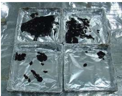
Fig. 1 Drained binder on the aluminum foil
