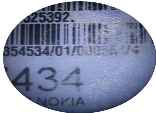
Fig. 2 Stereomicroscopic picture of enhanced IMEI
