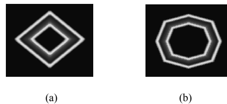
Fig. 11 ring pattern obtained by above method with N=10 , u_{up} = u_{Down} = 1 , u_2 = 0.2 and (a) \Delta = 2 (b) \Delta = 3 . Part b in this figure is more similar to fig. 1 (a) which is shown ideal ring pattern.
