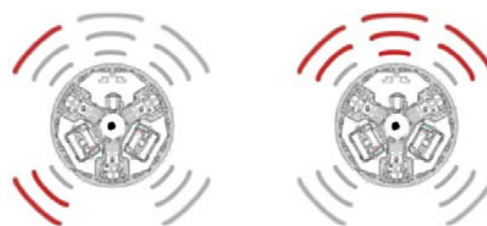
Fig. 8. Two examples of a metaphor for an intuitive representation of distance values. The visualization is in style of a parking distance control of a car. The center of each example shows a top view of the robot.
