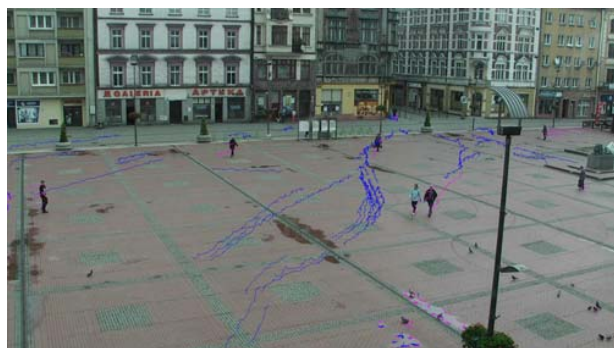
Fig. 4. Filtered set of tracks with the track length threshold equal to 50
