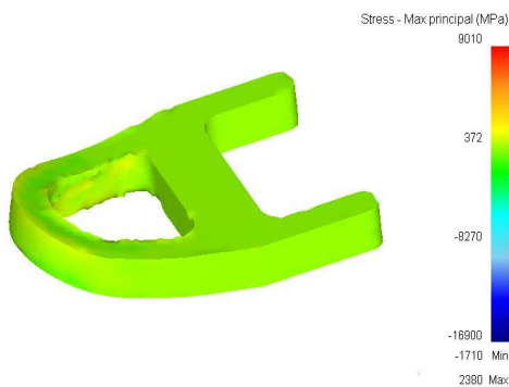
Fig. 6 Distribution of strain-max principal of professional bicycle pedal
