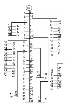
Fig. 1. 69-bus radial distribution system
