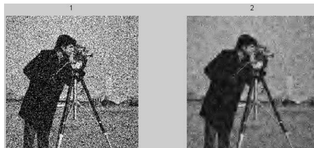
Fig. 5 1. Degraded image (blur + noise) 2. Multiscale Blind image restoration
