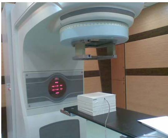
Fig. 2 set up for parallel-plate chamber measurements
