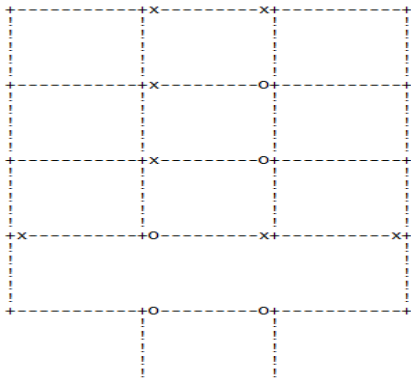
Fig. 4 Damaged state of floating column building
