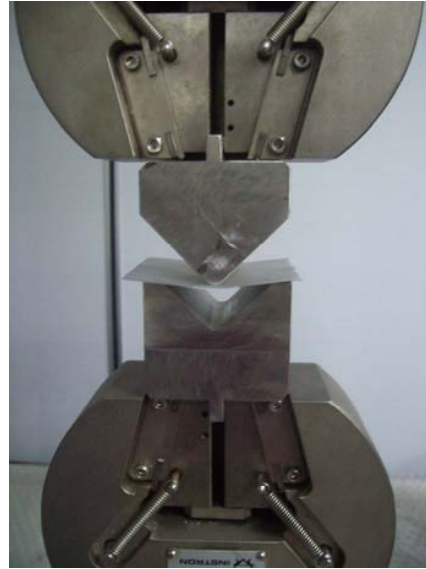
Fig. 2 Experimental set-up for V-bending process
