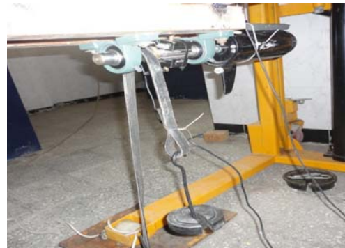
Fig. 5 Propeller torque measurement test rig
