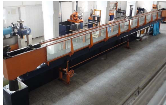
Fig. 2 Experimental water channel facility
