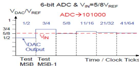
Fig. 3 Example of 6-bit SAR ADC [4]
