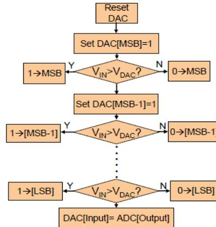
Fig. 1 SAR ADC algorithm block diagram [4]
