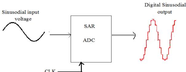
Fig. 6 Implemented SAR ADC Block diagram
