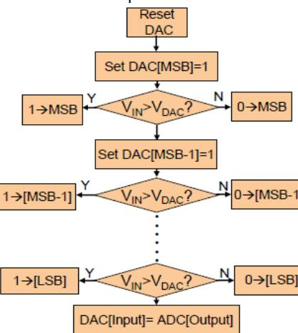
Fig. 1 SAR ADC algorithm block diagram [4]
