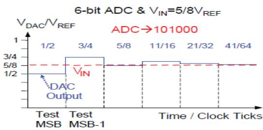
Fig. 3 Example of 6-bit SAR ADC [4]
