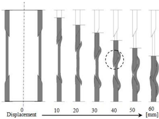
Fig. 18 Deformation diagram ( $t_2=3[\text{mm}]$ ,  $\delta=1.5t_2$  load)
