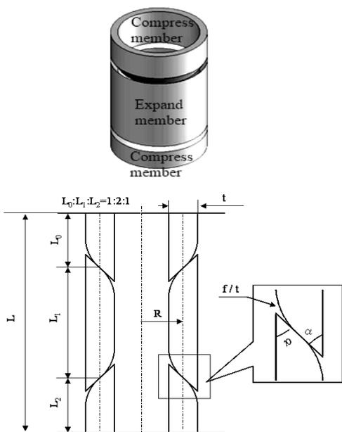
Fig. 2 Compress-expand member
