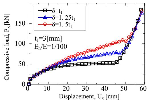
Fig. 17 Load-displacement curve with radius difference
