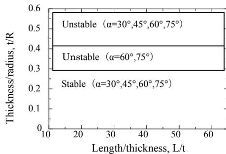
Fig. 15 Deformation modes distribution of contact angles
