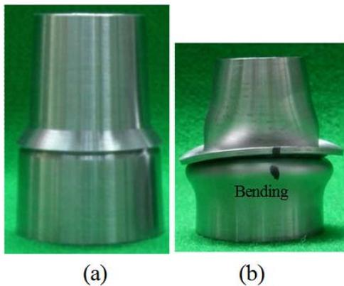
Fig. 5 Deformation of compress-expand member one
