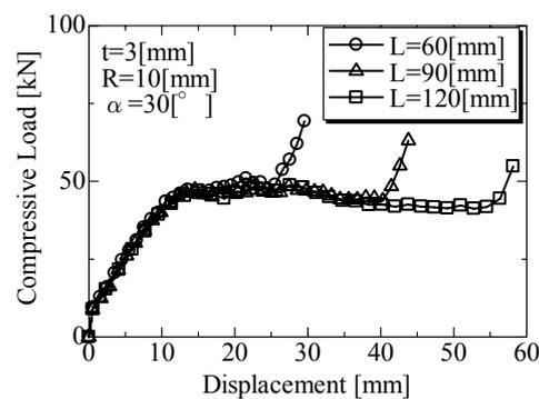
Fig. 10 Load-displacement curve for varied lengths
