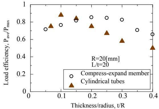
Fig. 13 Load efficiency for compress-expand member and circular tube
