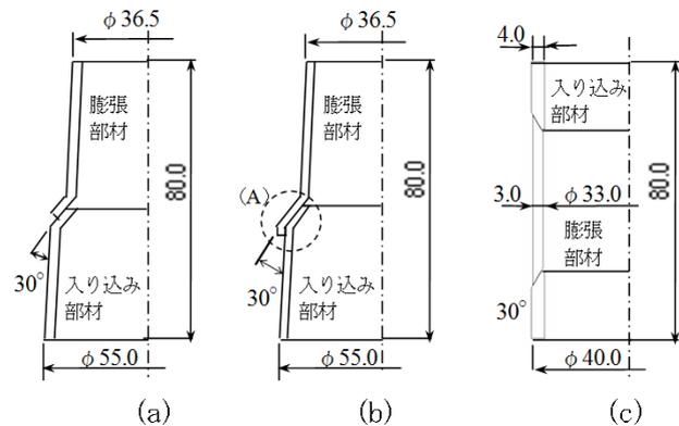
Fig. 3 Tube geometry and loading condition
