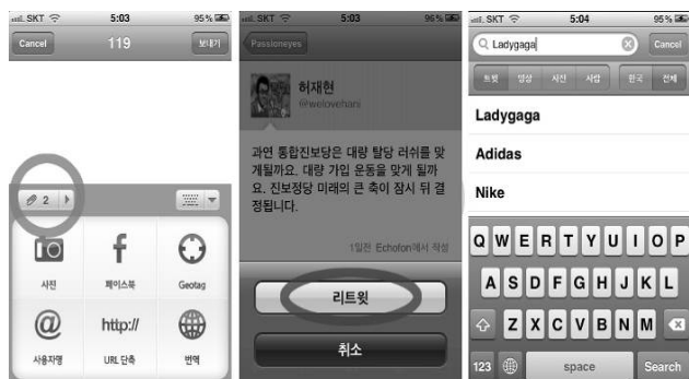
Fig. 14 (a) The number of attachments is marked, (b) Quotation Retweet function is excluded, (c) simplest interface of Search Tab
