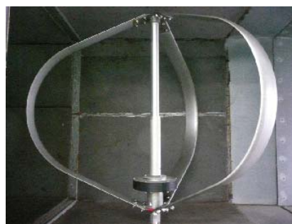
Fig. 2 Darrieus type VAWT for wind tunnel experiments
