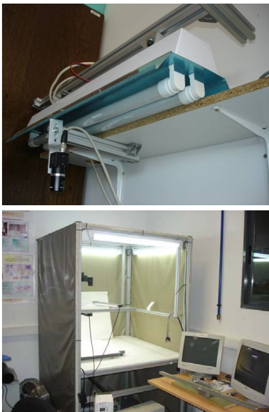
Fig. 3 Illumination testbed designed in the laboratory with fluorescent lamps, electronic ballasts and voltage regulators. The structure is closed to avoid external perturbation
