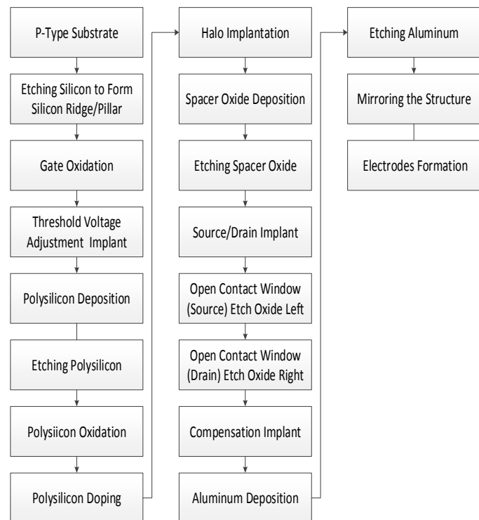
Fig. 2 Vertical DG-MOSFET's Process Simulation Flowchart
