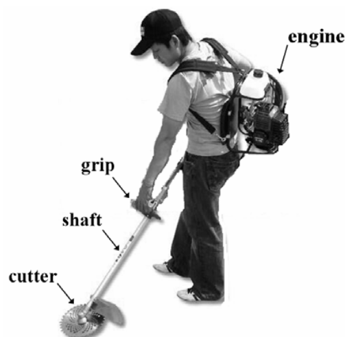
Fig. 1 Grass cutter and the name of each part
