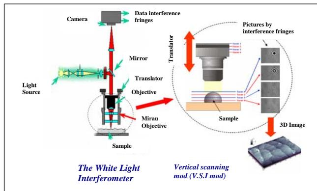
Fig. 6 Principle of interferometer [8].
