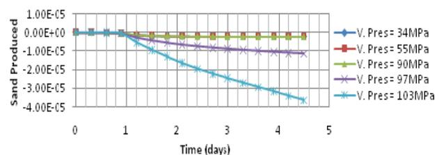
Fig. 1 Sand production with increasing vertical pressure
