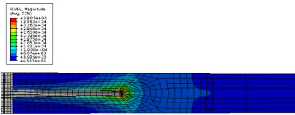
Fig. 6a Plot displaying higher pore fluid velocities at perf. tunnel dd=3.72MPa
