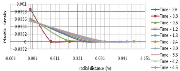
Fig. 4c Variation in plastic strain with time (DD=10.3MPa)
