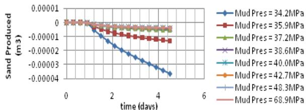
Fig. 9 Effect of mud pressure on sanding
