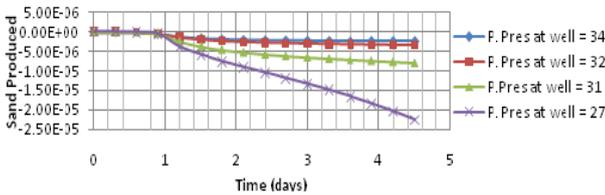
Fig. 3 Sand production with increasing constant drawdown
