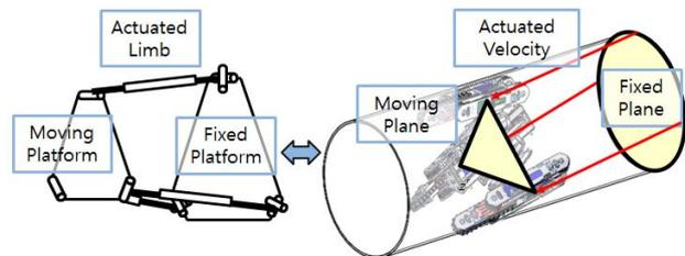
Fig. 2 Analogousness between parallel manipulator and three legged in-pipe robot
