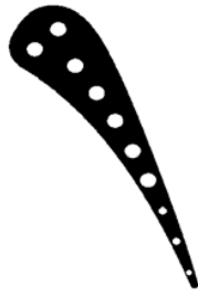
Fig. 1 C3X Vane with Cooling Holes
