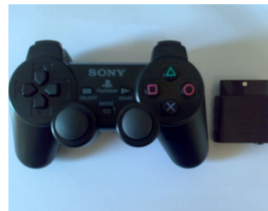
Fig. 4 Wireless PS2 Controller with Receiver
