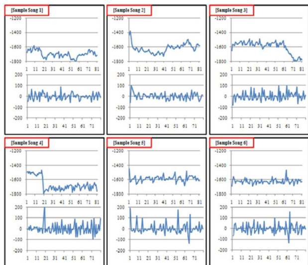
Fig. 2 Comparison of feature tendency of feature extracting steps. Each panel contains graphs of grouped MFCCs and delta-grouped MFCCs of 6 sample songs. The upper and lower graphs of each sample song show grouped MFCCs and delta-grouped MFCCs extracted from the sample, respectively. The song from sample song1 to sample song 6 is “She said she said” by the Beatles, “If i ain’t got you” by the Alicia Keys, “Into the new world” by the Girls generation, “Hungry spider” by the Makihara noriyuki, “Rak tae doo lae mai dee” by the Potato and “Je suis venue te dire que je m’en vais” by the Monica Nonueira, respectively.
