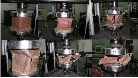
Fig. 8 Progress of Crashing Test of SQJFT
