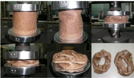
Fig. 9 Progress of Crashing Test of CJFT
