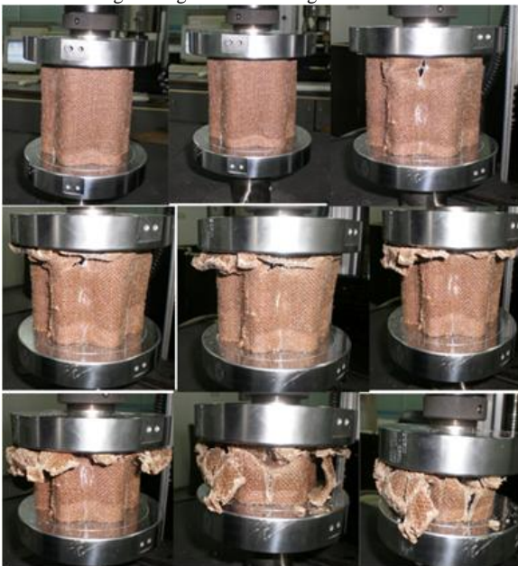
Fig.10 Progress of Crashing Test of RCJFT
