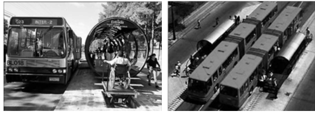
Fig. 4 Tube elevator for special needs users in Curitiba
