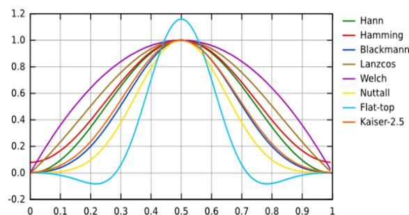
Fig. 4. The window functions used in speech processing
