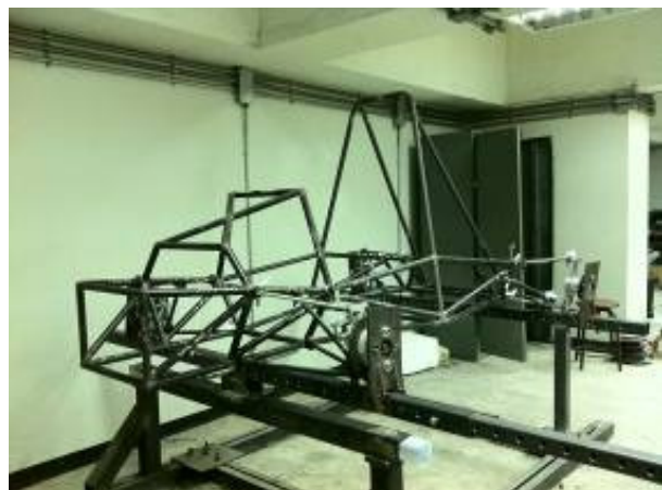
Fig. 20 Rapidamente's torsional stiffness test rig
