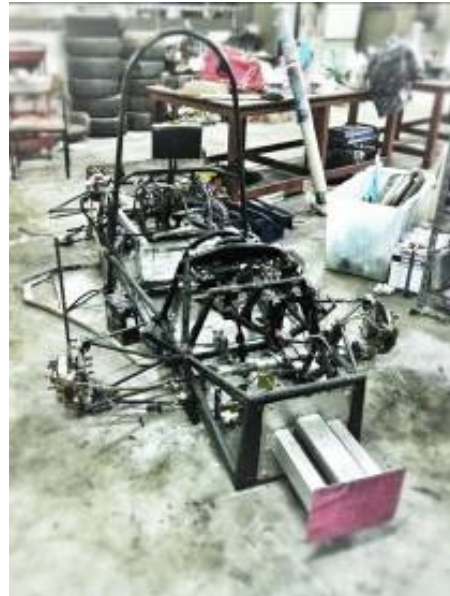
Fig. 12 Modified rapidamente91 student formula frame (cut off members)
