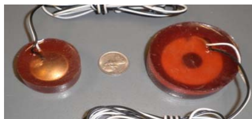
Fig. 1 Potted Transducers, DSTO-1 (see left), RING-1 (see right)
