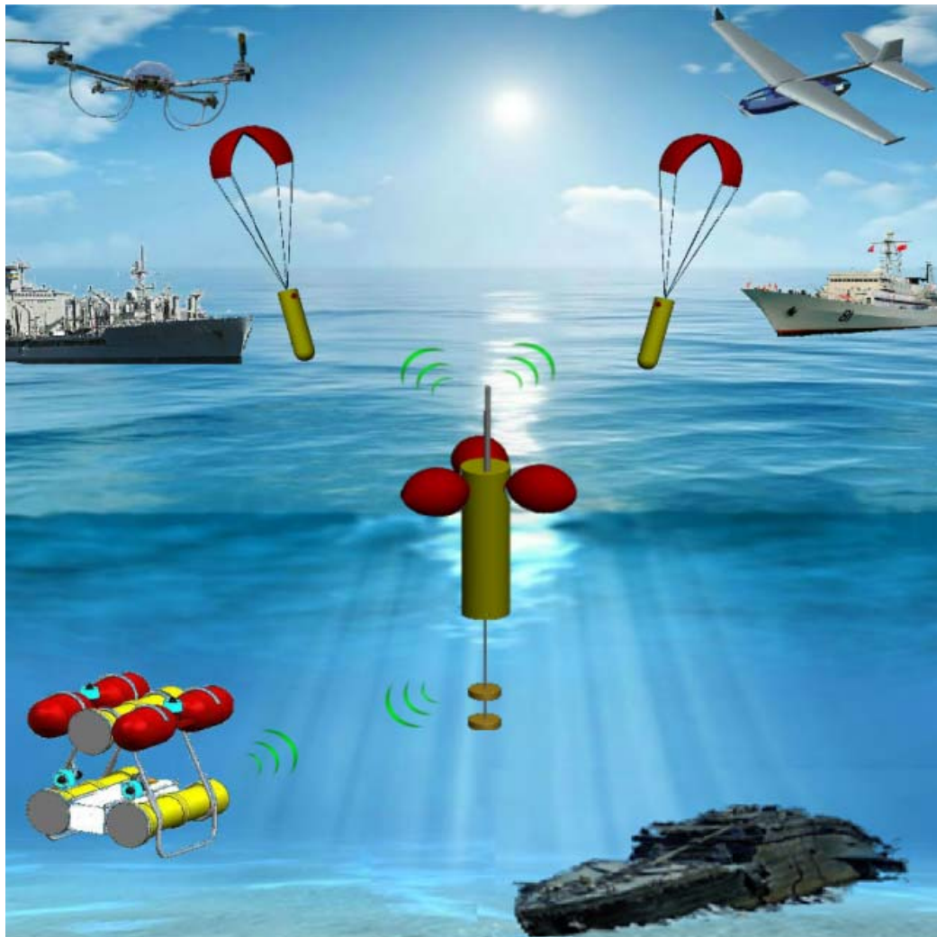
Fig. 4 Micro Communications Sonobuoy Deployment Phases
