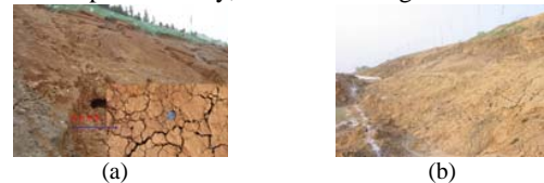
(a) Fractures of laterite (b) Shallow layer Landslide due to the dry-wet circulation Fig. 2 Common problems of fracturing laterite
