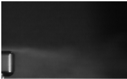
Fig.4 Wake in Smoke tunnel (Experiment)
