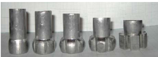
Fig. 14. Teeth formation stages for 3 and 6 teeth parts
