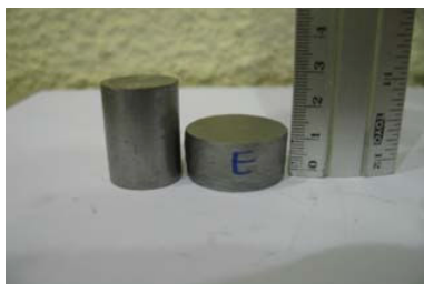
Fig. 2. Initial and final compressed lead specimen
