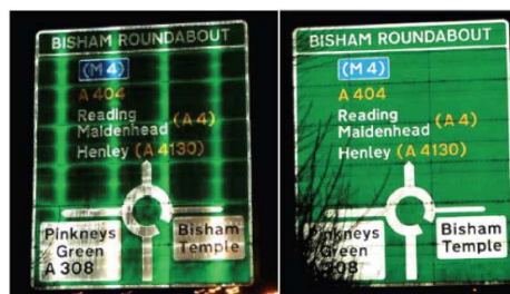
Fig. 4 The same sign photographed at night using the camera flash, in the presence (left) and absence (right) of dew [1]
