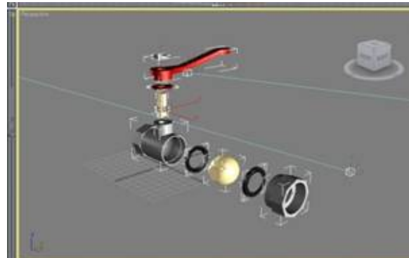
Fig. 4 Exploded view of Ball valve in 3DS Max
