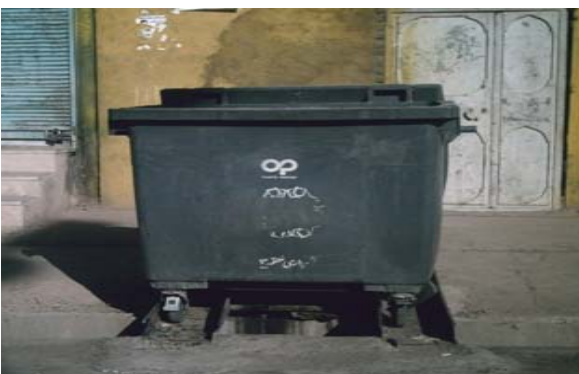
Fig. 4 Type of mechanical container for MSW collection in main streets and commercial areas, Khoram Abad
