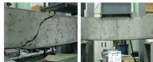
Fig. 15 Anchored titanium strengthened RC structure failure mode
