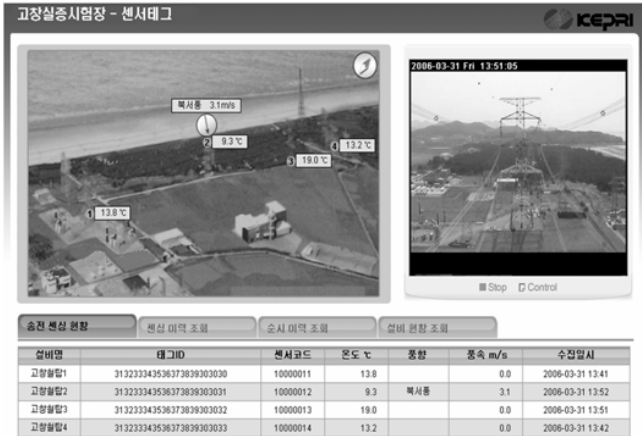
Fig. 5 Web screen of transmission tower monitoring system
