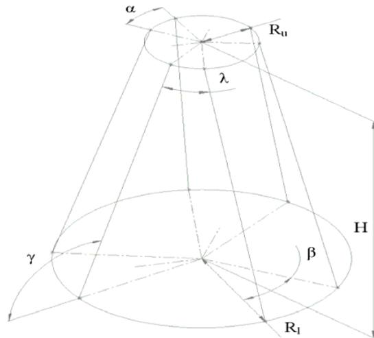
Fig. 2. Typical design parameters of a hexapod
