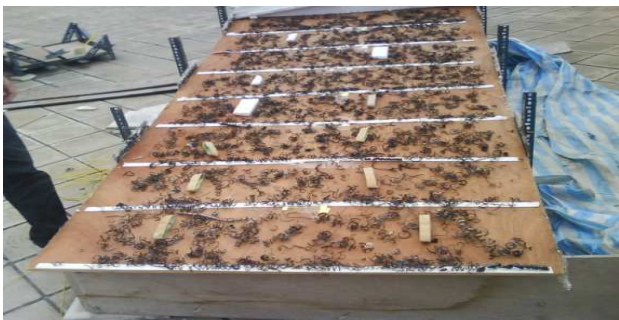
Fig. 15 Steel wire-stuffed channel (Case 5)
