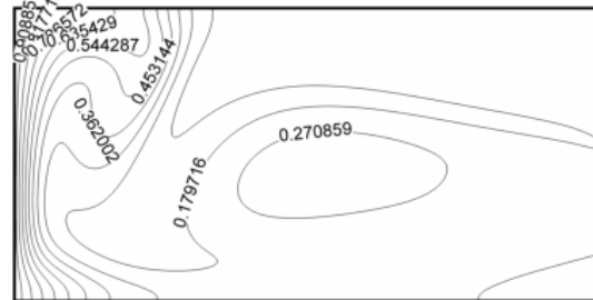
Fig.7 Streamline and Temperature contour for A=2,Ra=10 5 ,Pr=0.71, θ = 90
