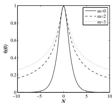
Fig. 8 Temperature at the fin tip ( $\theta_0$ ), as a function of  $N$  for  $m = 0, 2, 3$
