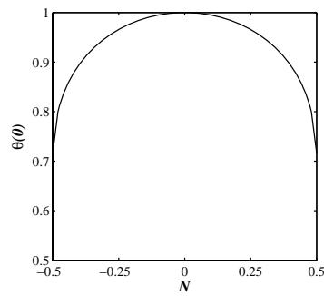
Fig. 6 Temperature at the fin tip ( $\bar{\theta}$ ), as a function of  $N$  for  $m = -4$
