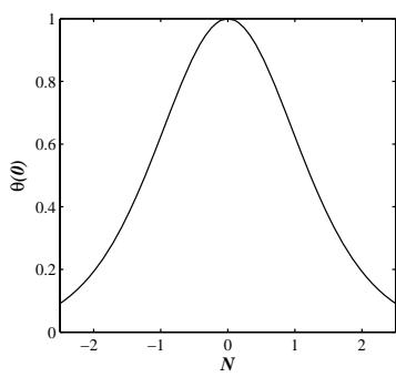
Fig. 7 Temperature at the fin tip ( $\bar{\theta}$ ), as a function of  $N$  for  $m = -0.25$
